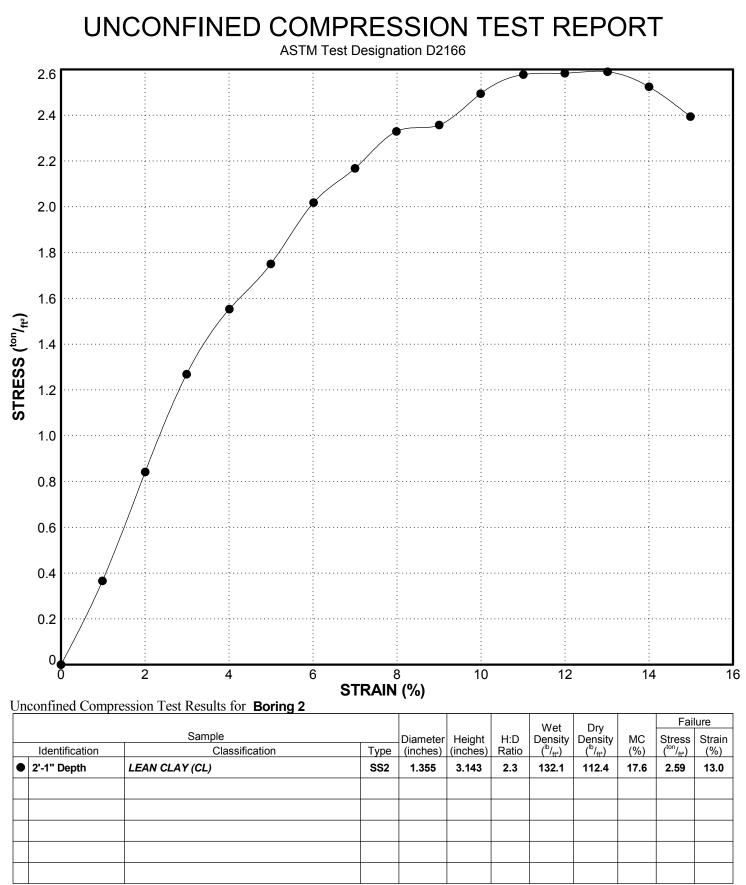
SS2=2-inch-outside-diameter, split-barrel sampler
